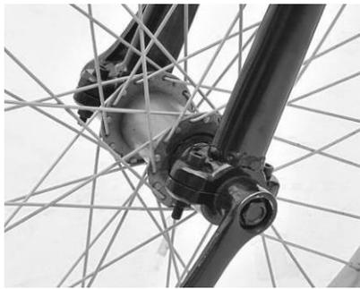
Insert front wheel assembly (part 3) into the open ends of the Front fork (part 2). Attach the two end covers and secure with bolt and nut (part 11)
