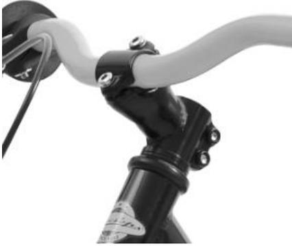
Insert the handlebar (4) into the stem clamp and secure by tightening the two Allen Bolts. Ensure the bolts are tightened evenly.
