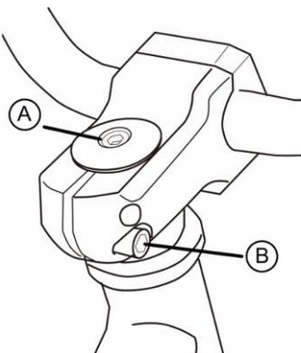
The stem is pre-assembled .If necessary, rotate the stem and fork to face the forward position. Ensure the stem is aligned with the front fork and facing the correct direction.
