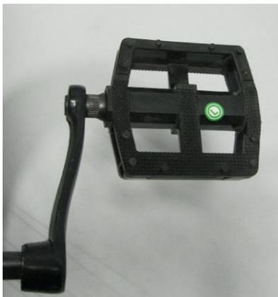
Attach the pedals (5) to the crank and tighten with spanner or adjustable wrench
