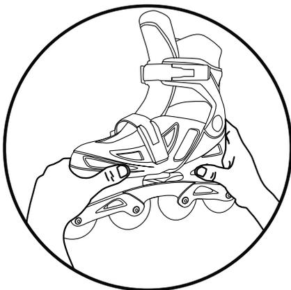
1. Press and hold the adjustable button then pull or push the toe to desired size then release the button with a "click"
