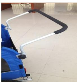
Remove the back portion of the top cover. Loosen both knobs on each side of the handle.
