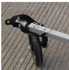
Remove the QR pin that attached on the hitch arm, and insert the swivel wheel stud of the wheel into the receiver. Replace and lock the QR pin, making sure the wheel is locked in place.
